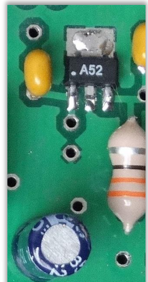
Fig. 30, Component side (RX preamp, SGA5289).
