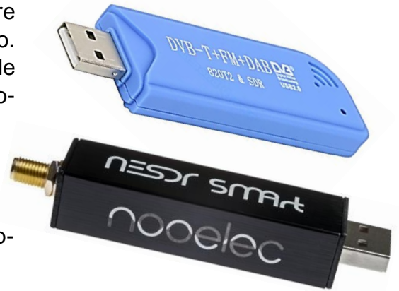
Figure 9, RTL-SDR USB sticks.
